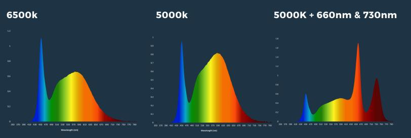
The LED tube is available in three different light recipes, 6500K for cloning cannabis, as well as 5000K and 5000K + 660nm & 730nm for greens and other vegetables. Tube lights are sold in packs of four to provide you with the coverage you need while saving on costs.
